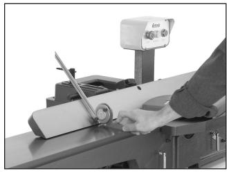
Figure 66. Adjusting fence 45° outward.
